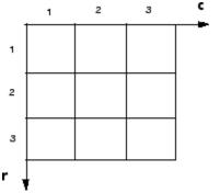
For pixel coordinates, the number of rows, r, downward, while the number of columns, c, increase to the right. Pixel coordinates are integer values and range from 1 to the length of the row or column. The pixel coordinates used in Computer Vision System Toolbox software are one-based, consistent with the pixel coordinates used by Image Processing Toolbox<sup>TM</sup> and MATLAB. For more information on the pixel coordinate system, see "Pixel Indices" (Image Processing Toolbox).
